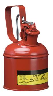
Dim.: 120 x 220 (dia x H in mm) interior tin plated exterior red powder coated Slef-closing opening stainless steel flame arrester in can neck Automatic pressure compensation Marking prepared according to GefStoffV and BGV A8
