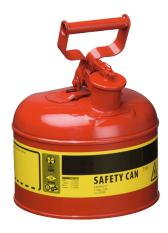
Dim.:  $185 \times 305$  (Dia x H in mm) interior tin plated exterior red powder coated Slef-closing opening Flame arrester in can neck Automatic pressure compensation Marking prepared according to GefStoffV and BGV A8
