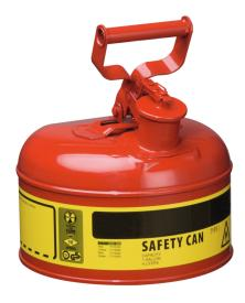
Dim.: 241 x 279 ( dia x H in mm ) interior tin plated exterior red powder coated Self-closing opening stainless steel flame arrester in can neck Automatic pressure compensation Marking prepared according to GefStoffV and BGV A8. Testings: FM, UL, TÜV-GS
