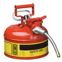
Sheet steel interior tin plated, exterior red powder coated, Self-closing opening, stainless steel flame arrester in can opening automatic pressure/vacuum compensation Dim.: 241 x 267 ( dia x H in mm ) galvanised metal hose, length: approx. 229 mm Diameter of hose: approx. 16 mm Marking prepared according to GefStoffV and BGV A8. Testings: FM, UL, TÜV-GS
