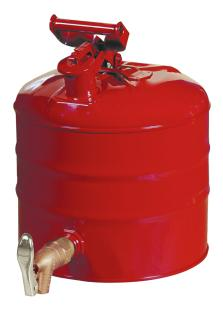
Sheet steel, interior tin plated Exterior red powder coated Dosing tap from brass Self-closing openings Flame arrester in can neck Automatic pressure/ vacuum compensation Dim.: 298 x 292 (Dia x H) mm Marking prepared according to GefStoffV and BGV A8 Testing: FM-approved
