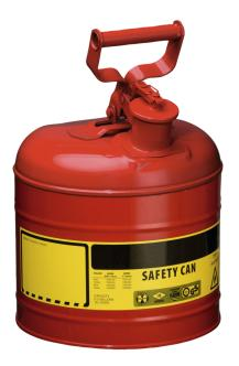
Dim.: 241 x 349 ( dia x H in mm ) interior tin plated exterior red powder coated Self-closing opening stainless steel flame arrester in can neck Automatic pressure compensation Marking prepared according to GefStoffV and BGV A8. Testings: FM, UL, TÜV-GS
