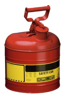
Dim.: 241 x 349 ( dia x H in mm ) interior tin plated exterior red powder coated Self-closing opening stainless steel flame arrester in can neck Automatic pressure compensation Marking prepared according to GefStoffV and BGV A8. Testings: FM, UL,  $T\ddot{U}V$ -GS
