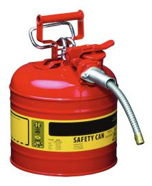
Sheet steel interior tin plated, exterior red powder coated, Self-closing opening, stainless steel flame arrester in can opening automatic pressure/vacuum compensation Dim.:  $241 \times 337$  ( dia x H in mm ) galvanised metal hose, length: approx. 229 mm Diameter of hose: approx. 16 mm Marking prepared according to GefStoffV and BGV A8. Testings: FM, UL, TÜV-GS
