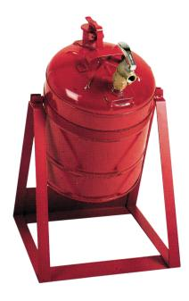
Consisting of: Tilt can 19 litres and framework rack can made from sheet steel, interior tin plated Exterior red powder coated Dosing tap from brass Self-closing openings Flame arrester in in filling opening Automatic pressure / vacuum compansation Tipping frame :  $365 \times 370 \times 600$  (L x W x H) mm Marking prepared according to GefStoffV and BGV A8 Testing: FM-approved
