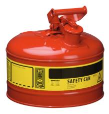
Dim.: 298 x 292 ( dia x H in mm ) interior tin plated exterior red powder coated Self-closing opening stainless steel flame arrester in can neck Automatic pressure compensation Marking prepared according to GefStoffV and BGV A8. Testings: FM, UL, TÜV-GS
