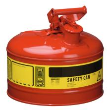
Dim.: 298 x 292 ( dia x H in mm ) interior tin plated exterior red powder coated Self-closing opening stainless steel flame arrester in can neck Automatic pressure compensation Marking prepared according to GefStoffV and BGV A8. Testings: FM, UL, TÜV-GS
