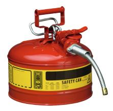
Sheet steel interior tin plated, exterior red powder coated, Self-closing opening, stainless steel flame arrester in can opening automatic pressure/vacuum compensation Dim.:  $298 \times 305$  ( dia x H in mm ) galvanised metal hose, length: approx. 229 mm Diameter of hose: approx. 16 mm Marking prepared according to GefStoffV and BGV A8. Testings: FM, UL, TÜV-GS
