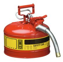
Sheet steel interior tin plated, exterior red powder coated, Self-closing opening, stainless steel flame arrester in can opening automatic pressure/vacuum compensation Dim.:  $298 \times 305$  ( dia x H in mm ) galvanised metal hose, length: approx. 229 mm Diameter of hose: approx. 25 mm Marking prepared according to GefStoffV and BGV A8. Testings: FM, UL, TÜV-GS
