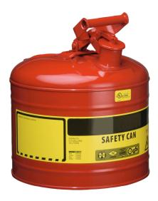
Dim.: 298 x 429 ( dia x H in mm ) interior tin plated exterior red powder coated Self-closing opening stainless steel flame arrester in can neck Automatic pressure compensation Marking prepared according to GefStoffV and BGV A8. Testings: FM, UL, TÜV-GS
