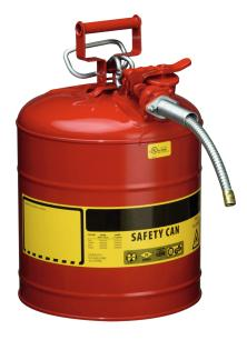
Sheet steel interior tin plated, exterior red powder coated, Self-closing opening, stainless steel flame arrester in can opening automatic pressure/vacuum compensation Dim.: 298 x 445 ( dia x H in mm ) galvanised metal hose, length: approx. 229 mm Diameter of hose: approx. 16 mm Marking prepared according to GefStoffV and BGV A8. Testings: FM, UL, TÜV-GS
