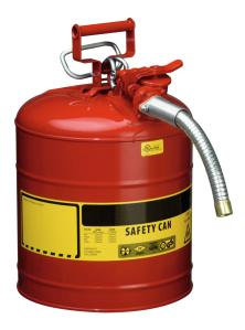
Sheet steel interior tin plated, exterior red powder coated, Self-closing opening, stainless steel flame arrester in can opening automatic pressure/vacuum compensation Dim.: 298 x 445 ( dia x H in mm ) galvanised metal hose, length: approx. 229 mm Diameter of hose: approx. 25 mm Marking prepared according to GefStoffV and BGV A8. Testings: FM, UL, TÜV-GS
