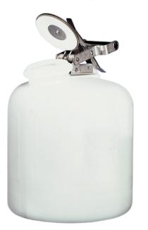
FOR NON-FLAMMABLE LIQUIDS Dimensions: 260 x 370 (Dia x H) mm Self-closing opening without flame arrester Dispensing parts-Material made from stainless steel Automatic pressure compensation Marking prepared meeting GefStoffV and BGV A8
