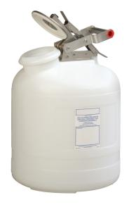
FOR NON-FLAMMABLE LIQUIDS Dimensions: 310  $\times$  450 (Dia  $\times$  H) mm Self-closing opening big charging hole without flame arrester Dispensing parts-material made from stainless steel Automatic pressure compensation Marking prepared meeting GefStoffV and BGV A8
