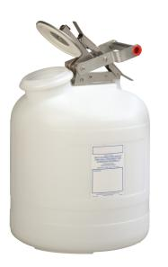
FOR NON-FLAMMABLE LIQUIDS Dimensions: 310 x 450 (Dia x H) mm Self-closing opening big charging hole without flame arrester Dispensing parts-material made from stainless steel Automatic pressure compensation Marking prepared meeting GefStoffV and BGV A8
