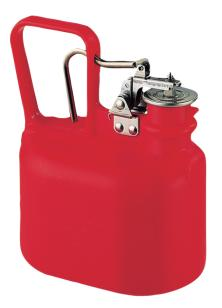
Dim: 140 x 200 x 240 (W x D x H) mm Self-closing lid incl. flame arrester in charging hole fittings and flame arrester made from stainless steel Automatic pressure compensation Marking prepared according to GefStoffV and BGV A8 Tested safety product testing: FM-approved
