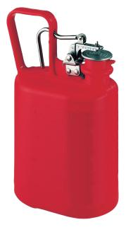
Dim:  $140 \times 200 \times 330$  ( W x D x H ) mm Self-closing lid incl. flame arrester in charging hole fittings and flame arrester made from stainless steel Automatic pressure compensation Marking prepared according to GefStoffV and BGV A8 Tested safety product testing: FM-approved
