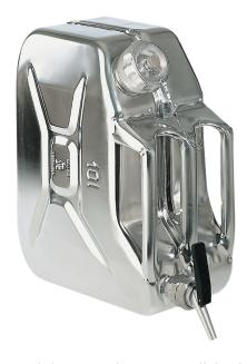
stainless steel 1.4301 polished Dim:  $175 \times 350 \times 300$  (W x D x H) mm 3/4 connection ( for tap optional) flame arrester in screw cap Manual pressure / vacuum compensation in screw cap Markings prepared according to StoffV and BGV A8
