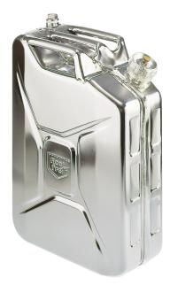
stainless steel 1.4301 polished Dim:  $175 \times 350 \times 490$  (W x D x H) mm 3/4 connection ( for tap optional) flame arrester in screw cap Manual pressure / vacuum compensation in screw cap Markings prepared according to StoffV and BGV A8
