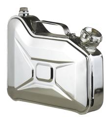
stainless steel 1.4301 l polished Dim:  $105 \times 350 \times 300$  (W x D x H) mm 3/4 "- connection ( for tap optional) flame arrester in screw cap Manual pressure / vacuum compensation in screw cap Markings prepared according to StoffV and BGV A8
