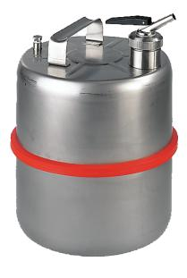
Stainless steel 1.4571 unpolished Dim. 260 x 340 (dia x H) mm Flame arrester in can neck Self-closing metering tap with ventilation Manual vacuum compensation/ overpressure compensation Markings prepared according to GefSoffV and BGV A8
