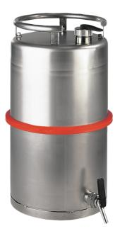
Unpolished stainles steel 1.4301 Dim: 300 x 530 (dia x H ) mm with revolving carry handle, stackable Flame arrester in can neck manual pressure/vacuum compensation in the screw cap Selfclosing tap Markings prepared according to GefStoffV and BGV A8
