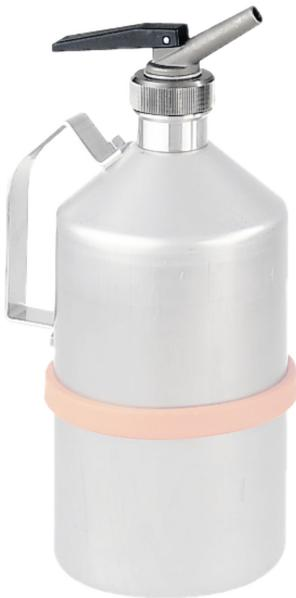
Unpolished stainless steel 1.4301 Dim: 300 x 530 (dia x H ) mm with revolving carry handle, stackable Flame arrester in can neck manual pressure/vacuum compensation in the screw cap Self-closing tap Markings prepared according to GefStoffV and BGV A8
