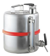
Unpolished, stainless steel 1.4571 Dim. 260 x 330 (dia x H) mm level indicator made from PFA Flame arrester in can neck Self-closing metering tap Manual pressure/vacuum compensation in the screw cap Markings prepared according to GefSoffV and BGV A8
