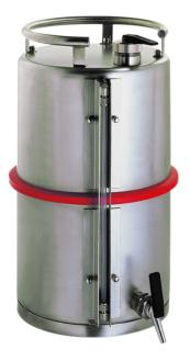
Unpolished, stainles steel 1.4301 Dim: 300 x 530 (dia x H ) mm level indicator made from PFA Flame arrester in can neck Self-closing metering tap Manual pressure/vacuum compensation in the screw cap Markings prepared according to GefSoffV and BGV A8
