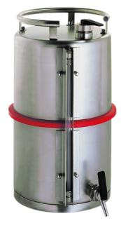
Unpolished, stainles steel 1.4301 Dim:  $300 \times 530$  (dia x H ) mm level indicator made from PFA Flame arrester in can neck Self-closing metering tap Manual pressure/vacuum compensation in the screw cap Markings prepared according to GefSoffV and BGV A8
