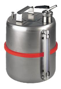
Unpolished, stainless steel 1.4571 Dim. 260 x 340 (dia x H) mm level indicator made from PFA Flame arrester in can neck Self-closing metering tap with ventilation Manual vacuum compensation/ overpressure compensation Markings prepared according to GefSoffV and BGV A8
