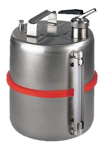
Unpolished, stainless steel 1.4571 Dim.  $260 \times 340$  (dia x H) mm level indicator made from PFA Flame arrester in can neck Self-closing metering tap with ventilation Manual vacuum compensation/ overpressure compensation Markings prepared according to GefSoffV and BGV A8
