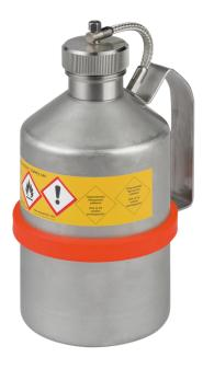
Unpolished stainless steel 1.4571 Dim:  $110 \times 238$  (dia x H ) mm Tigth closure, Captive cap on flexible shaft Flame arrester in can neck Type approval tested can according to ADR, RID and IMDG code Markings prepared according to GefStoffV and BGV A8 Aditional markings according to ADR/RID Testing: BAM-admittance
