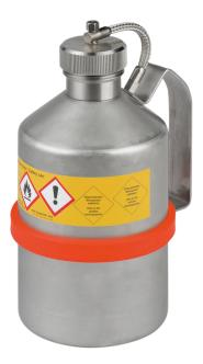
Unpolished stainless steel 1.4571 Dim: 110 x 238 (dia x H ) mm Tigth closure, Captive cap on flexible shaft Flame arrester in can neck Type approval tested can according to ADR, RID and IMDG code Markings prepared according to GefStoffV and BGV A8 Aditional markings according to ADR/RID Testing: BAM-admittance
