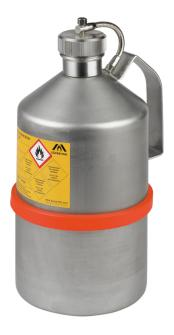
Unpolished stainless steel 1.4571 Dim: 130 x 270 (dia x H ) mm Tigth closure, Captive cap on flexible shaft Flame arrester in can neck Type approval tested can according to ADR, RID and IMDG code Markings prepared according to GefStoffV and BGV A8 Aditional markings according to ADR/RID Testing: BAM-admittance
