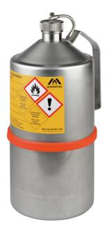
Unpolished, stainless steel 1.4571 Dim: 165 x 380 (dia x H ) mm Tigth closure, Captive cap on flexible shaft Flame arrester in can neck Type approval tested can according to ADR, RID and IMDG code Markings prepared according to GefStoffV and BGV A8 Aditional markings according to ADR/RID Testing: BAM-admittance
