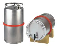
stainless steel 1.4301, unpolished Dimensions: 300 x 530 (Dia x H) mm Plastic protection ring, stockable tight closure, manual ventilation captive cap on flexible shaft flame arrester in can neck Container constructed according to ADR, RID, IMDG Cording and ICAO-TI Marking prepared meeting GefStoffV an BGV A8 and ADR/RID Testing: BAM-admittance
