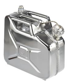
stainless steel 1.4301, polished Dim: approx. 105 x 350 x 300 (W x D x H) mm Adjusting bases for stable positioning Rear handle 3/4 '' connection, tight closure, Captive cap on flexible shaft. Flame arrester in container neck. Type approval tested can according to ADR, RID and IMDG code and ICAO-TI. Marking prepared according to GefStoffV and BGV A8 tested: BAM-approval
