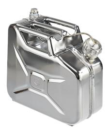
stainless steel 1.4301, polished Dim: approx.  $105 \times 350 \times 300$  (W x D x H ) mm Adjusting bases for stable positioning Rear handle 3/4 " connection, tight closure, Captive cap on flexible shaft. Flame arrester in container neck. Type approval tested can according to ADR, RID and IMDG code and ICAO-TI. Marking prepared according to GefStoffV and BGV A8 tested: BAM-approval
