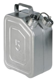
Stainless steel 1.4571, polished Dim:approx.130 x 210 x 290 (W x D x H in mm) Tight closure, Captive cap on flexible shaft Flame arrester in container neck Type approval tested can according to ADR, RID, IMDG code. Markings prepared according to GefStoffV and BGV A8 and ADR / RID. testing: BAM-approval
