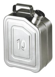
Stainless steel 1.4571, polished Dim:approx. 130 x 280 x 370 ( W x D x H ) mm Tight closure, Captive cap on flexible shaft, Flame arrester in container neck Type approval tested can according to ADR, RID, IMDG code, Markings prepared according to GefStoffV and BGV A8 and ADR/RID. testing: BAM-approval
