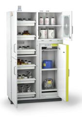
consisting of 1 CLASSIC standard S: Type 90, safety cabinet with wing door. for the storage of flammable liquids Type-tested by MPA/ TÜV SÜD according to DIN EN 14470-1, DIN EN 16121, and DIN EN 16122, EK5/AK4 09-10:2009 and AfPS GS 2014: 01 PAK mark of approval: GS/CE mark, high quality mark of approval by TÜV SÜD fittings and features:
