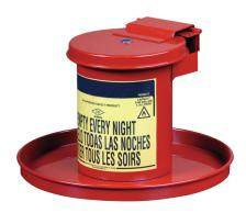
Dim.: approx. 267 x 178 (D x H in mm), outside powder coated red, inside tin-plated Self-closing lid after usage. Markings prepared according to GefStoffV and BGV A 8. Testing: FM/UL-approved
