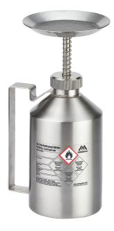
Stainless steel 1.4571 (AISI 316Ti) polished Dimensions: approx. 105 x 273 mm (dia x H) without srew cap. Flame arrester in container neck, Markin prepared according to GefStoffV including soaking tray with flame arrester and pump tube stainless steel 1.4301
