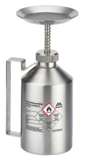
Stainless steel 1.4571 (AISI 316Ti) polished Dimensions: approx. 105 x 273 mm (dia x H) without srew cap. Flame arrester in container neck, Markin prepared according to GefStoffV including soaking tray with flame arrester and pump tube stainless steel 1.4301
