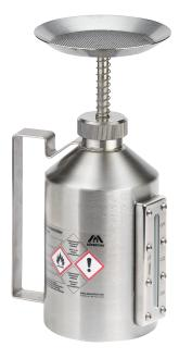
Stainless steel 1.4571 (AISI 316Ti) polished Dimensions: approx. 105 x 273 mm (dia x H) without srew cap. Flame arrester in container neck, Level control via integrated sight glass with measuring scale. Markin prepared according to GefStoffV including soaking tray with flame arrester and pump tube stainless steel 1.4301
