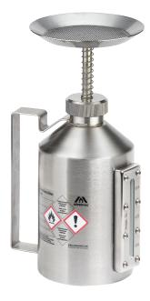
Stainless steel 1.4571 (AISI 316Ti) polished Dimensions: approx.  $105 \times 273 \text{ mm}$  (dia x H) without srew cap. Flame arrester in container neck, Level control via integrated sight glass with measuring scale. Markin prepared according to GefStoffV including soaking tray with flame arrester and pump tube stainless steel 1.4301
