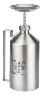
Stainless steel 1.4571 (AISI 316Ti) polished Dimensions: approx. 120 x 333 mm (dia x H) without srew cap. Flame arrester in container neck, Markin prepared according to GefStoffV including soaking tray with flame arrester and pump tube stainless steel 1.4301
