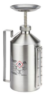
Stainless steel 1.4571 (AISI 316Ti) polished Dimensions: approx. 120 x 333 mm (dia x H) without srew cap. Flame arrester in container neck, Level control via integrated sight glass with measuring scale. Markin prepared according to GefStoffV including soaking tray with flame arrester and pump tube stainless steel 1.4301
