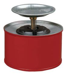
Dimensions:  $180 \times 145$  ( dia x H in mm). Soaking tray: 135 mm dia, interior tin plated, exterior red powder coated, soaking tray with flame arrester, brass pump tube and PPS. Marking prepared according to GefStoffV and BGV A8. testing: FM-tested
